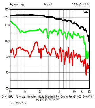
**Figure 11. Response and Distortion - Beryllium Diaphragm.** (Fundamental-Black; 2<sup>nd</sup> Harmonic-Green; 3<sup>rd</sup> Harmonic-Red)
