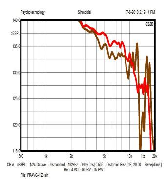
Figure 14. Response of Beryllium (red) vs Ribbed Titanium (brown) Diaphragm.
